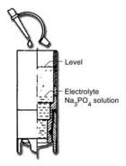
Unscrew the probe's head and the membrane permeable to oxygen.
