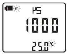
To manually change the compensation temperature press the °C/°F key once: the indicated temperature value starts blinking. Select the desired temperature value by using the arrows and confirm with ENTER. The display stops blinking, and the temperature displayed is used for compensation. To change the unit of measurement between °C and °F, press the °C/°F key **twice**.
