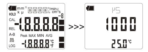
During turning on, should no probes be connected, the last manually-set temperature appears in the secondary line. The unit of measurement symbol (°C or °F) starts blinking, and a letter "m" meaning "manual" appears next to the battery symbol.
