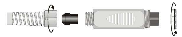
Open the two module shells: the printed circuit to which the temperature probe must be connected is housed inside. The wires coming from the conductivity cell are welded directly onto the connector's pins.
