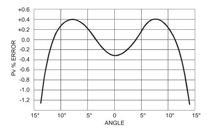
The abscissas reports the rotation angle around its vertical axis compared to the flow direction (yawing), in ordinates the % error on the differential pressure Pv measurement. As you can see a difference of over  $10^\circ$  entails an error on the differential pressure Pv measurement of less than 0.5%.
