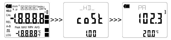
If no thermocouple probe is connected to the input, it is the manual temperature which is displayed in the secondary line. This value is 25°C by default.
