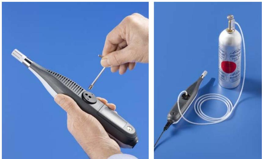
2. Let the inlet open if you want to perform a calibration at 400 ppm: For this second calibration procedure, **ensure the instrument is really in clean air.**
