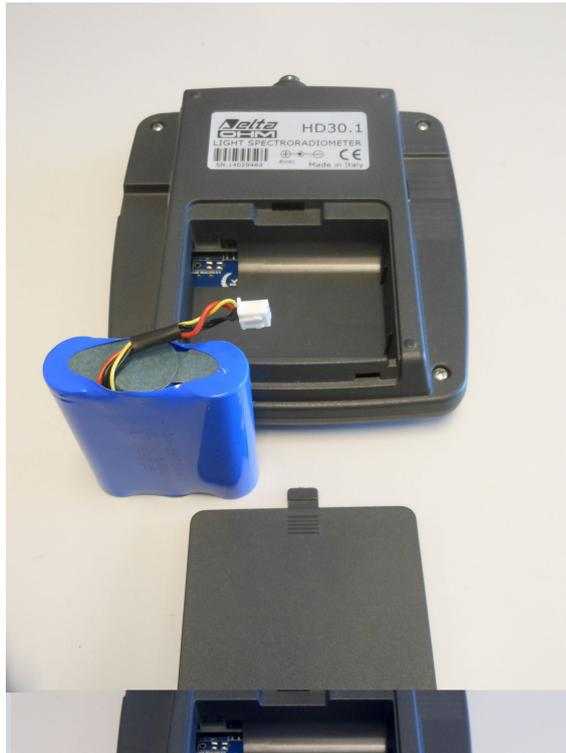
*Figure 2.2: Battery removed from housing.*
