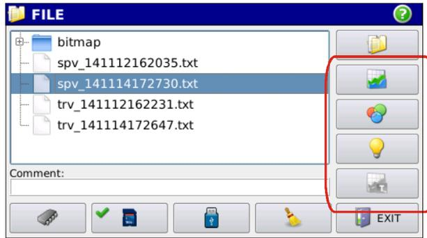
Fig. 4.12: Data contained into selected file can be displayed by using the highlighted keys.
