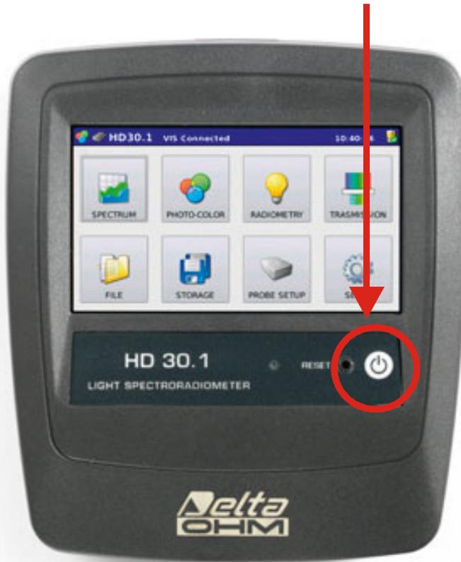
*Fig. 6.4 : Monitor reactivation button*
