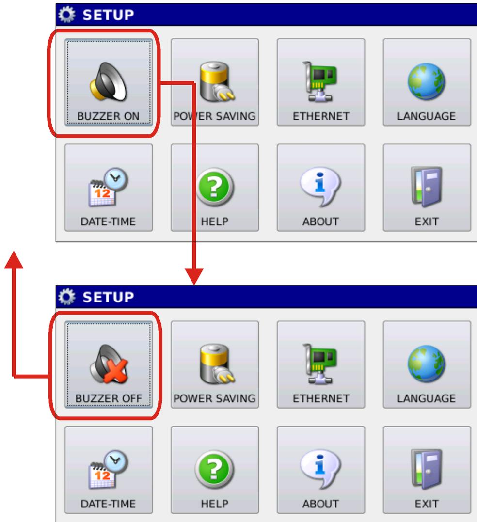
Fig. 6.2: Activating/deactivating acoustic signals through Buzzer key.
