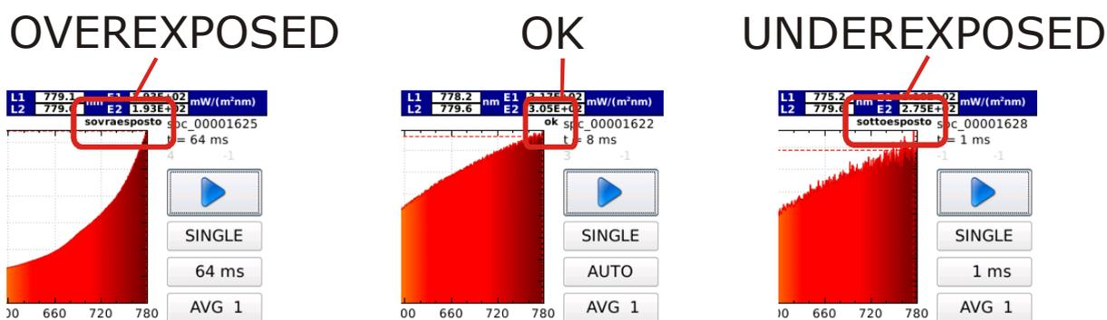
Figure 3.6: correct exposure time is displayed on top of graph.
