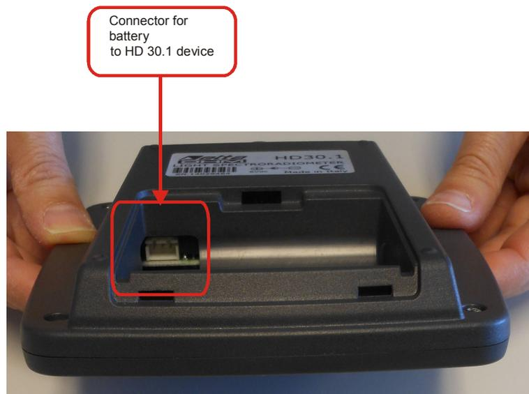
*Figure 2.3: Battery connector on HD 30.1 device*
