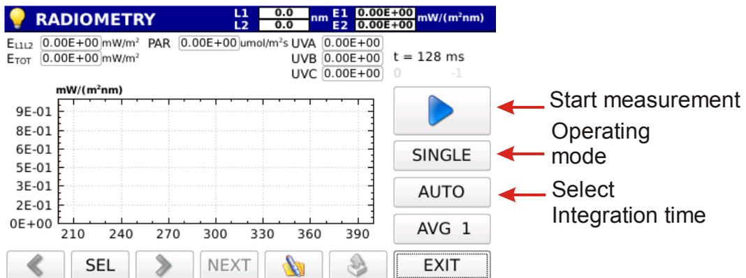
Fig3.17 Start-up screen in radiometry mode
