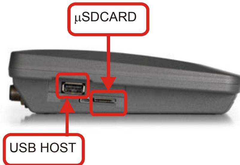
*Figure 10.2: Connectors for  $\mu$ SDCARD and USB HOST.*
