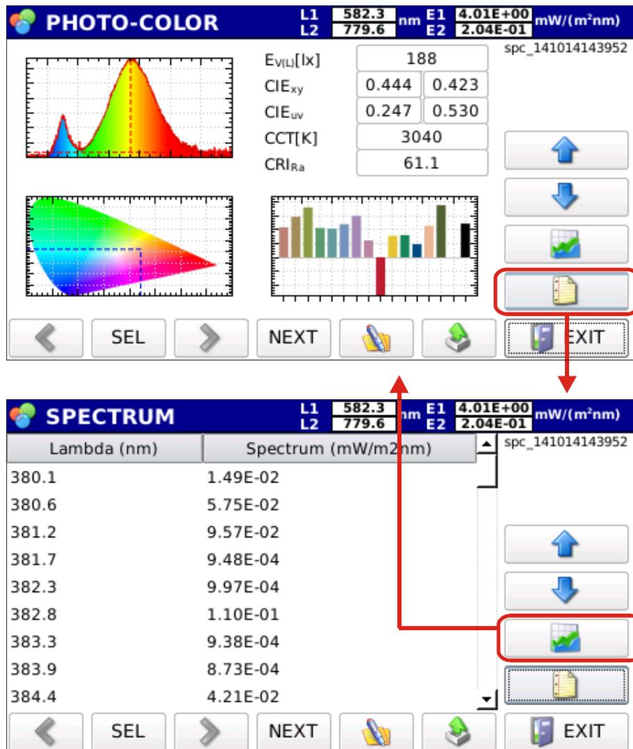
Fig. 4.17: Spectral irradiance data in text format
