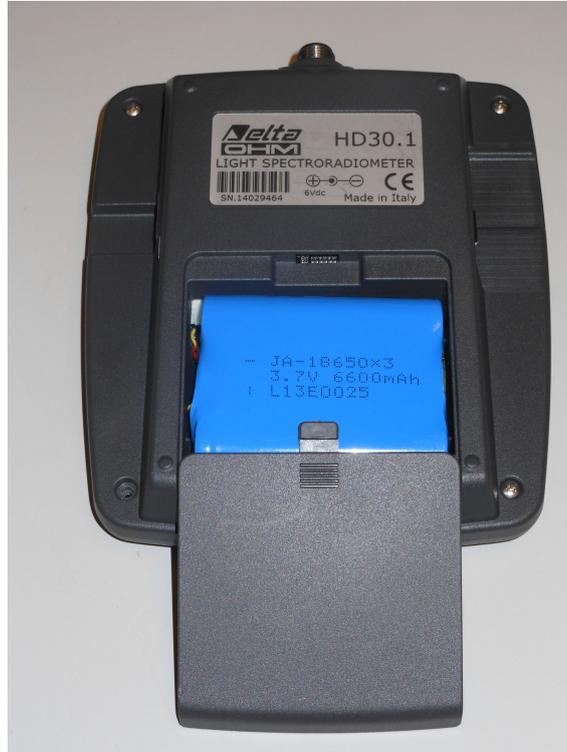
*Figure 2.1: Disconnected battery inside battery compartment.*
