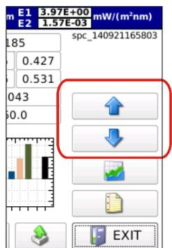
Fig. 4.14 : Arrow keys can be used to display files stored in memory.
