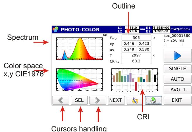
Figure 3.13: Example of screen in Photo-color measuring mode after measurement completion.
