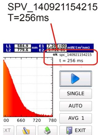
Figure 3.8: Data concerning file and integration time are shown on top right of the screen.
