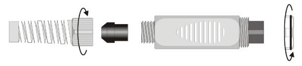
Open the two module shells: the printed circuit to which the probe must be connected is housed inside. On the left there are the 1...4 points on which the sensor wires must be welded. The JP1...JP4 jumpers are in the center of the board. For the 4-wire Pt100 sensor the jumpers must be left open.
