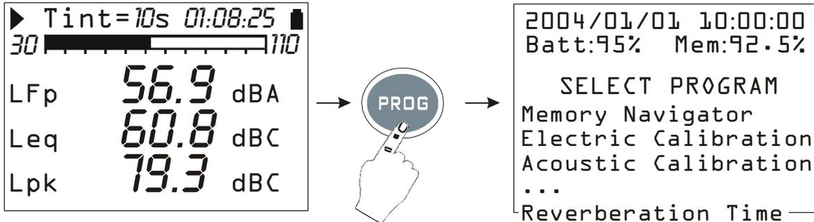
By using the arrows select the program "Reverberation Time" and confirm with **SELECT**<sup>3</sup>.
