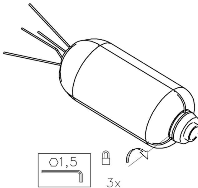
4. Insert the preamplifier (A) into the support pushing slowly upward until it's limit position.
