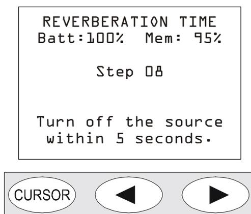
Now turn the sound source off **within 5 seconds**: the sound level meter will automatically measure the environment noise decay and will perform the calculations. For the entire duration of the measurement (6 seconds from the source being turned off) avoid undesired noises that could affect the measurement. The following page will appear at the end:
