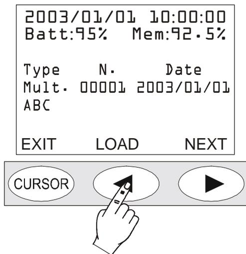
The following data are indicated for each file: the type (single, multiple, automatic or reverberation), the progressive number given by the instrument upon logging and the date. Press NEXT to jump to the next file, press LOAD to download the current file. If you press LOAD, the instrument goes back to standard display and the STOP and battery symbols alternate with the R (Replay) and P (Program) letters respectively.
