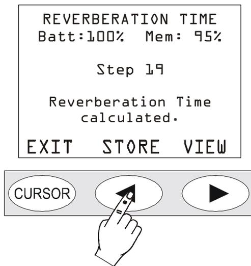
**To restore the standard SLM mode of the sound level meter and to exit the reverberation time measurement program, turn off the instrument (ON/OFF button) and then turn it back on.**
