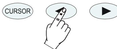
6. At the end, if the values of the electrical calibration are acceptable, press YES to confirm the new calibration (LEFT arrow of the keypad); press NO if you want to cancel the whole calibration (RIGHT arrow of the keypad).
