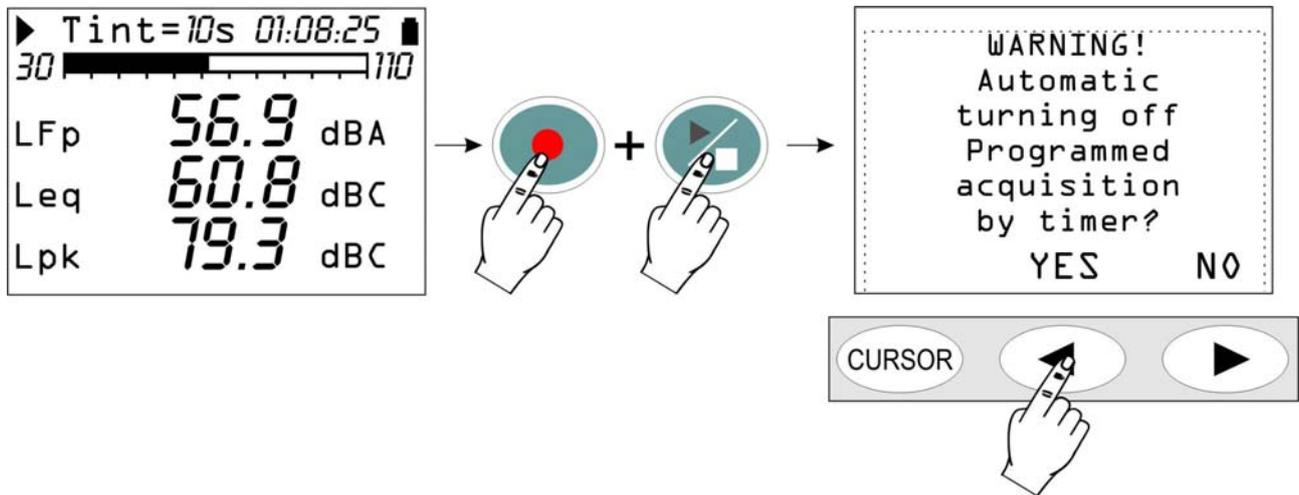
**Fig. 14 - Delayed acquisition timer warning screen**
