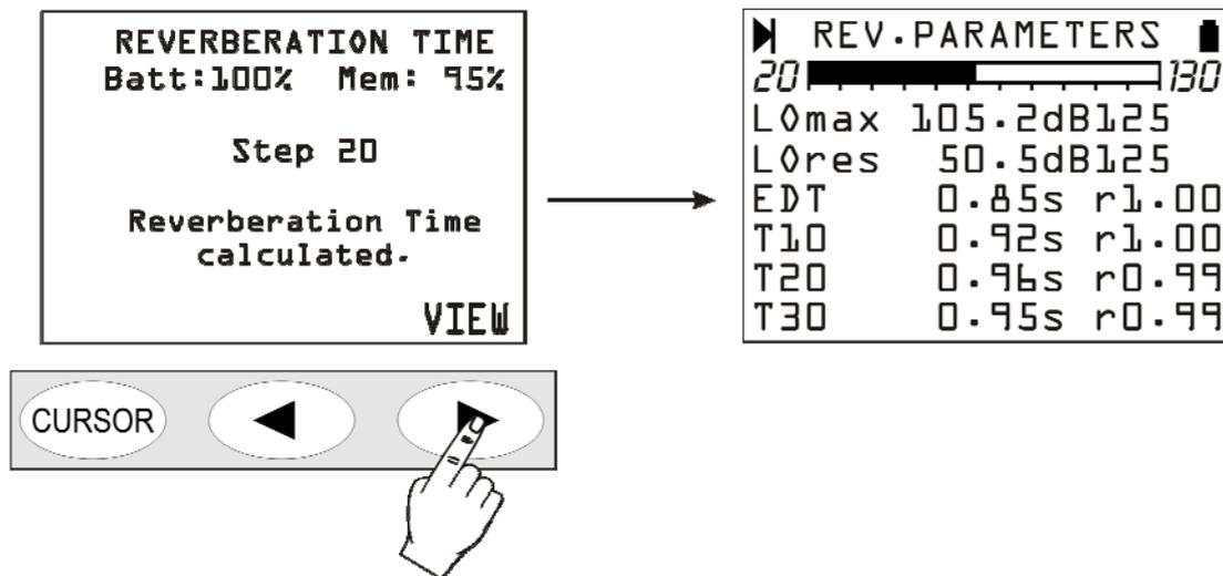
The sound level meter gives a complete description of the measurement both in the form of a table and graphically. See the paragraph describing the results: *"Reverberation Time - Analysis of the Results"*.
