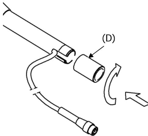
8. To secure the outdoor protection you can use the threaded end (D) or you can apply the fitting (E) on the tripod. The terminal (E) has two threads, 1/2 " and 1/4".
