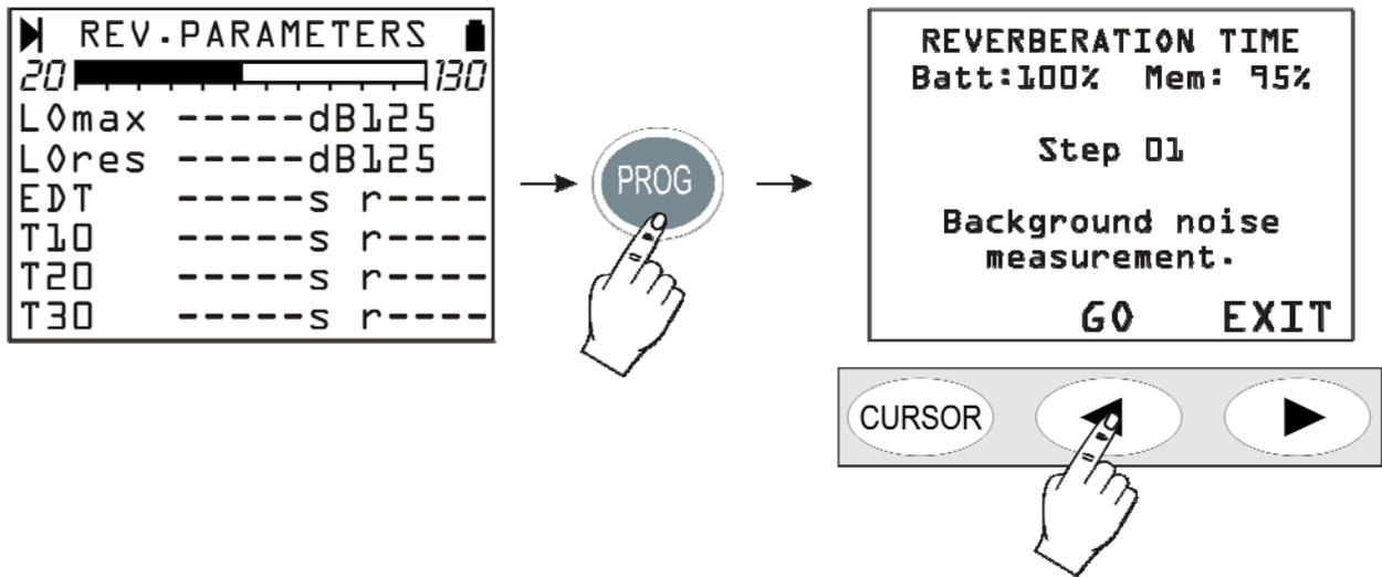
The current noise level is recorded and integrated for two seconds and then saved in the sound level meter internal memory.
