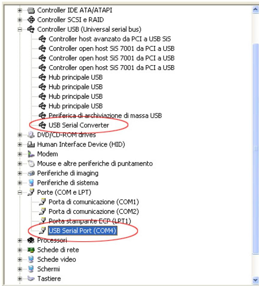
When USB cable is unplugged, the above items will disappear and they will appear again as soon as the instrument is plugged to USB port.
