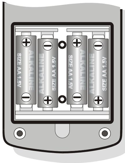
As an alternative to alkaline batteries, you can use rechargeable batteries. Batteries with lower capacity usually show greater impedance, causing a worsening of the electrical noise generated by the sound level meter, with repercussions on the measurement dynamic. Therefore zinc-carbon and rechargeable NiCd batteries are not recommended.
