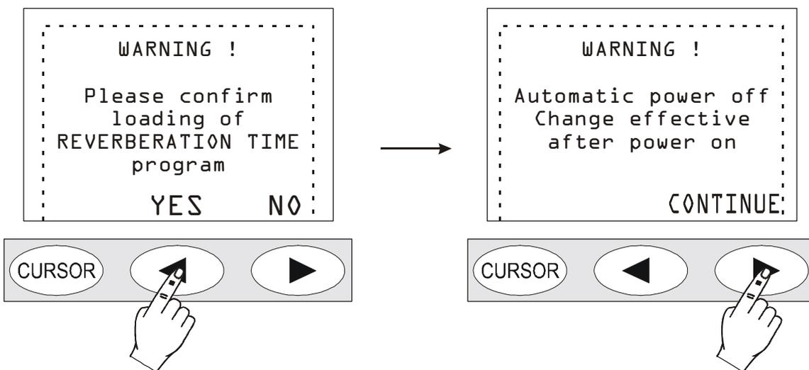
The sound level meter will automatically turn off.
