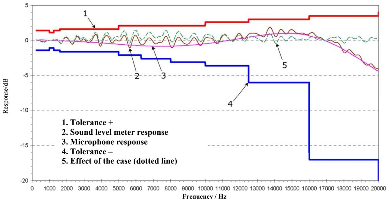
The selection of the UC52 microphones, on the basis of frequency response specifications, and the spectral corrections calculated by the sound level meter DSP allows obtaining a Class 1 response according to IEC61672:2002. The HD2010UC/A is also available in the Class 2 version.
