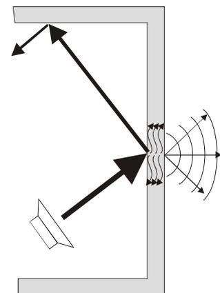
The absorption and the acoustic transmission is responsible for the progressive reduction of the sound wave at each interaction with the wall materials. Consequently, when the sound source is interrupted, after some time sound is no longer perceptible. The sound level will be maintained infinitely after the interruption of the sound source in an hypothetical room having walls with no absorption or transmission.
