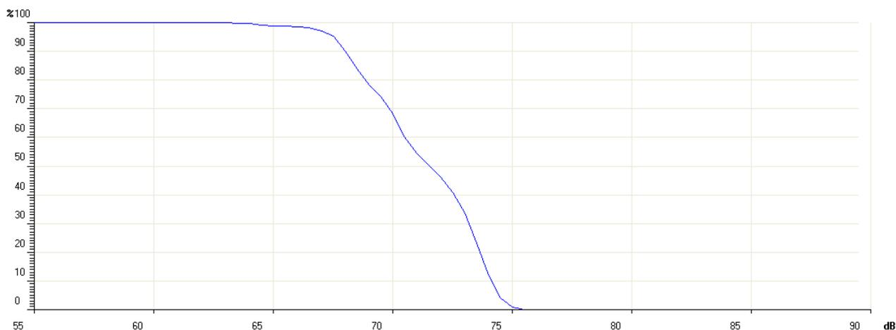
The cumulative probability will be null for levels higher than the maximum measured level. The percentile levels are calculated interpolating the cumulative distribution. For example, if from the analysis of the noise of a traffic road you detect that, the sound level (usually A weighted, examining the auditory impact), remains higher than 74dB half the time, the percentile level  $L_{50}$  is 74dB.
