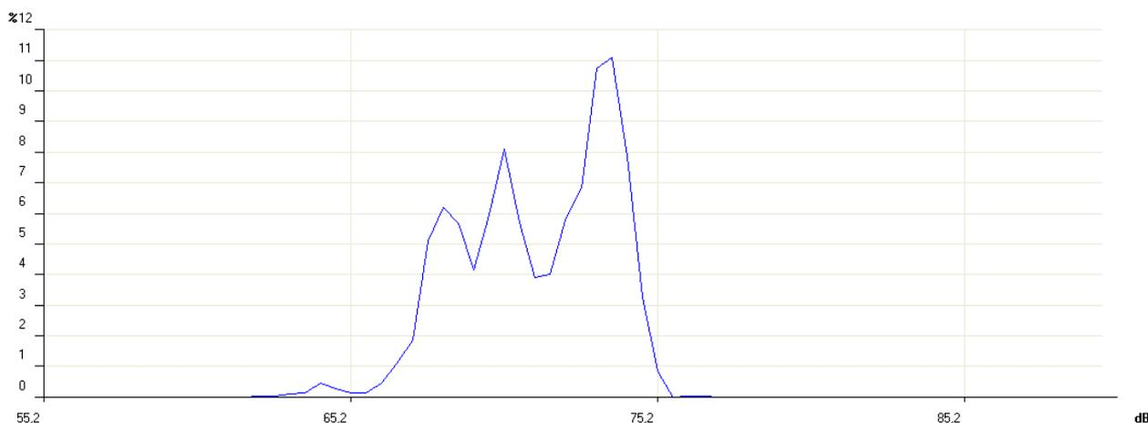
After this, the cumulative distribution is calculated. This is based on the sound level distribution of probabilities, beginning with a 100% probability for all lower classes with a value lower than the minimum measured level and for each class progressively subtracting the corresponding distribution probability of the level probabilities.
