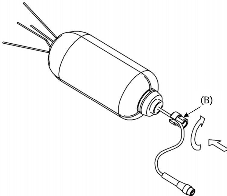
6. Insert the cable connected to the preamplifier through the system (C) and screw the stem to the support.
