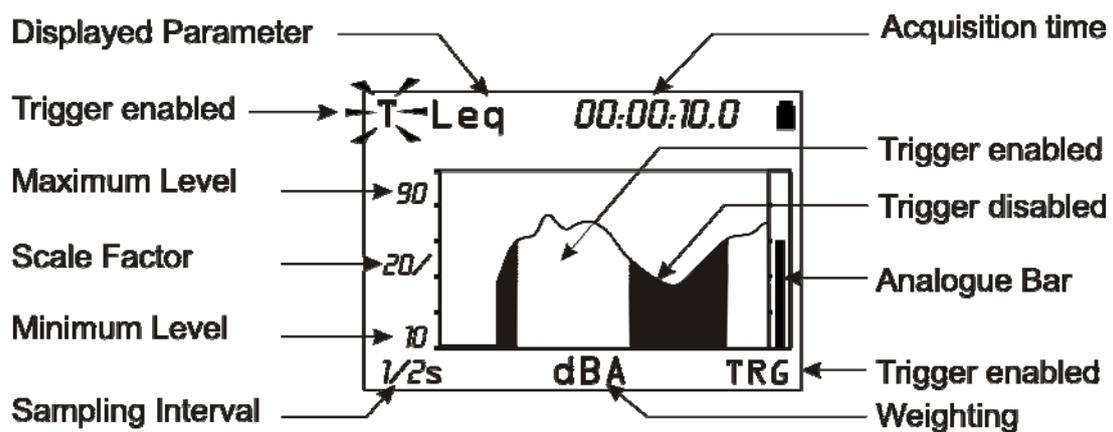
Fig. 11 - Description of the "Event trigger" display
