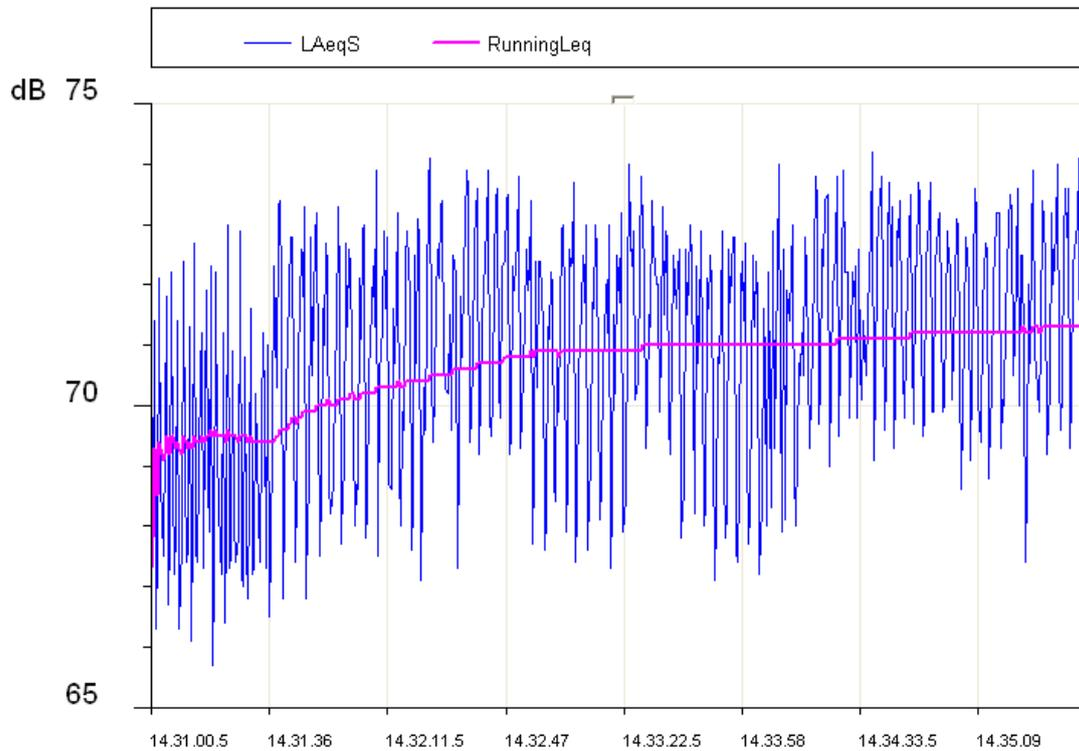
In the figure, the equivalent level profile is highlighted. It is stabilizing within few minutes to a level just above 71dBA.
