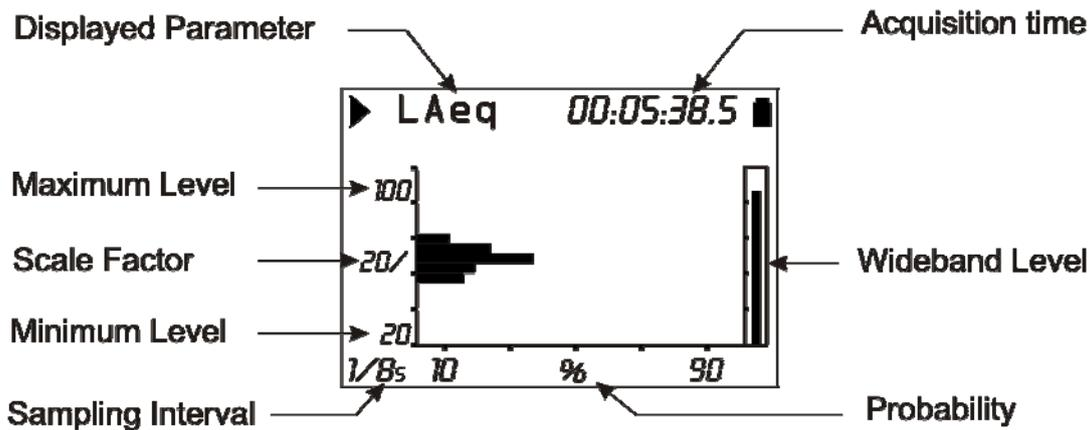
**Fig. 8 - Description of the distribution of probabilities display**
