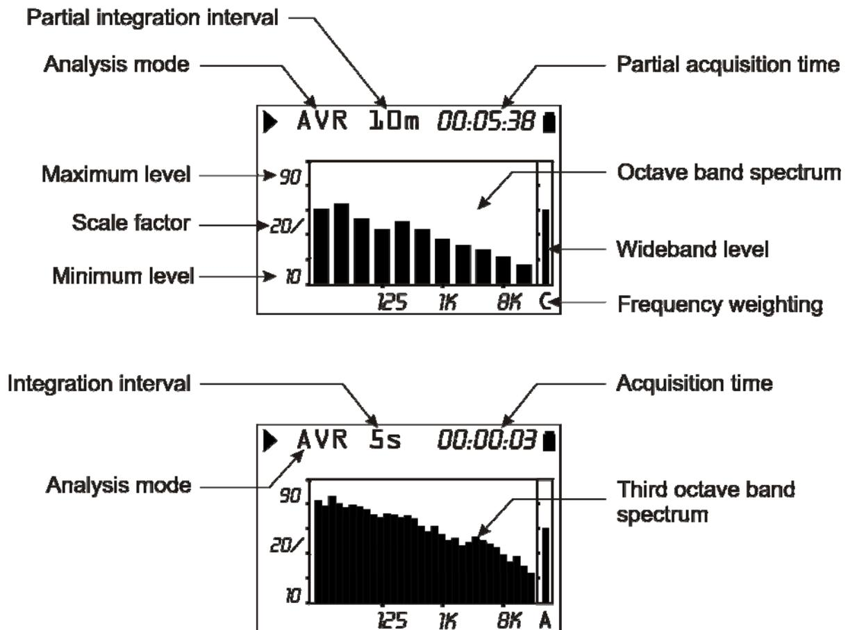
Spectral analysis, normally frequency unweighted (Z), can be carried out applying A or C frequency networks. The A or C frequency weighted analysis is used to evaluate audibility of different spectral components.
