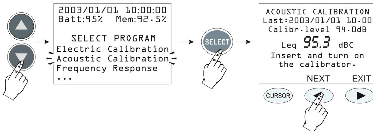
2. The first screen shows the date of the last calibration (Date:...) and, in the line below, the calibrator sound level to be used in the calibration in progress (this value can be modified, before starting the calibration program, by selecting "Calibration Level" from the MENU: see page.44). Gently insert the microphone in the calibrator hole and switch it on.
