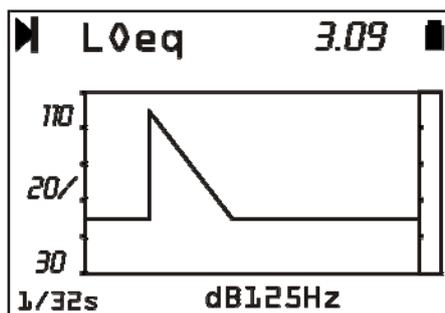
The upper number on the right (3.09) indicates the time in seconds in correspondence of the right border of the visible window of the graph. When the cursors are **not** active, you can move the graph horizontally on the time axis using the arrows. This function helps examine the decay profile when the measurement is taken in wide spaces where the reverberation time is longer than three seconds.
