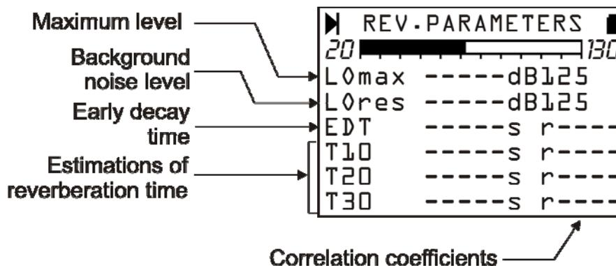
From top to bottom are shown: the maximum level in octave bands reached by the noise source (LO max), the background noise level in octave bands (LO res), the Early Decay Time EDT and the three estimations of the reverberation time  $T_{10}$ ,  $T_{20}$  and  $T_{30}$  each with the correlation coefficient “r”.
