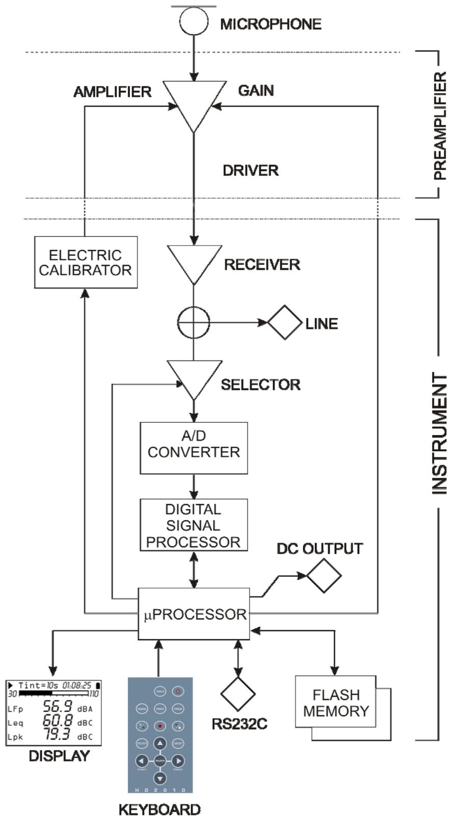
The block diagram shows the main elements of the HD2010UC/A sound level meter.
