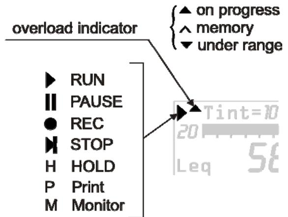
Just on the right of the symbol indicating the logging mode, there is the symbol showing a possible **overload** or under-range. An arrow directed upwards indicates that the input level has exceeded the maximum measurable level, while an arrow directed downwards indicates that the input level is lower than the minimum measurable level.
