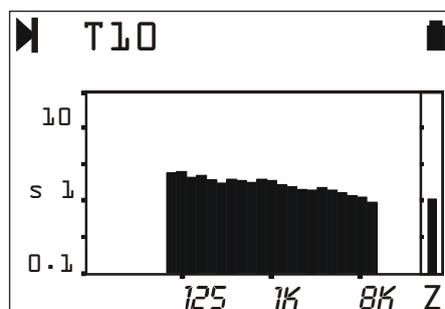
The variable ( $T_{10}$ ,  $T_{20}$ ,  $T_{30}$  or  $EDT$ ) are selected as usual by **SELECT** and the arrows: upon confirmation by pressing **ENTER**, the page is refreshed to show the new results.
