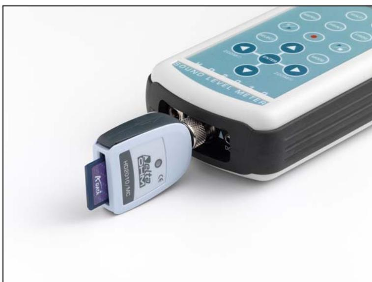
3. Insert the memory card in the slot of HD2010MC interface.
