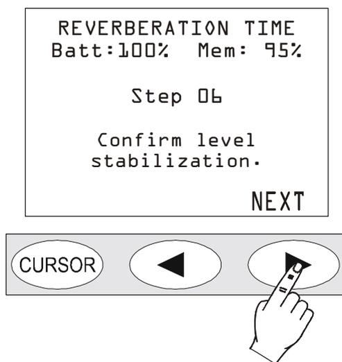
Wait until, according to the environment dimensions, the sound of the source stabilizes. Usually 4-5 seconds are enough even for wider environments, then proceed pressing the NEXT key.
