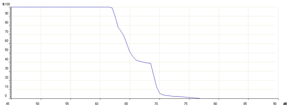
The *percentile levels* are calculated interpolating the cumulative distribution.
