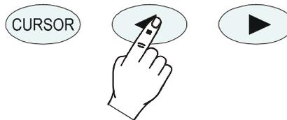
7. Press YES (keypad LEFT key) to confirm or NO (keypad RIGHT key) to refuse the calibration just finished. At the end, the instrument will switch to the SLM display, in STOP mode.
