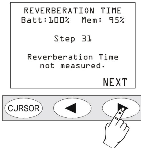
The same message is displayed if the signal/noise ratio between the generated signal and the background noise is not large enough.
