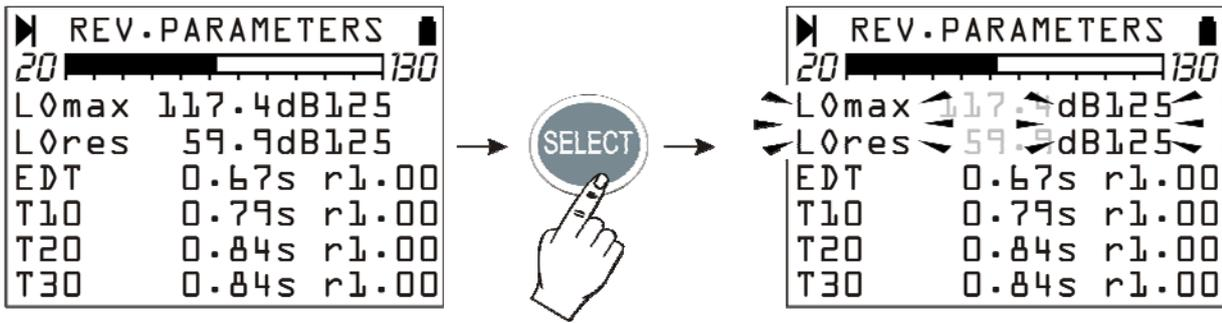
Confirm the selection by pressing the ENTER key. The sound level meter will calculate the new values and update the page showing the results.
