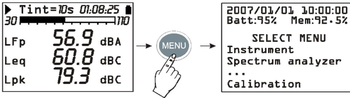
When you access the menus, current date and time are displayed, as well as the battery charge level and the available memory.
