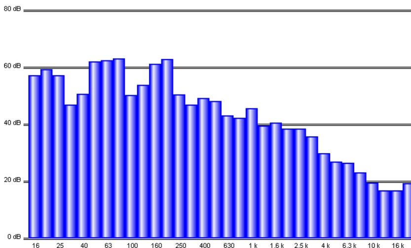
For example, the band centered at 1 kHz will consider the sounds between 707 Hz and 1414 Hz for octave and between 891 Hz and 1122 Hz for third octave bands. The analysis result is usually shown in a graph called “spectrogram” where the sound levels are represented in graphic format for each of the bands in which the sound spectrum
