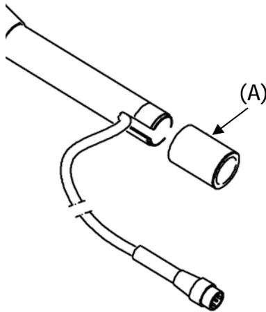
4. Unscrew the stem (B) and disconnect the cable connected to the preamplifier.
