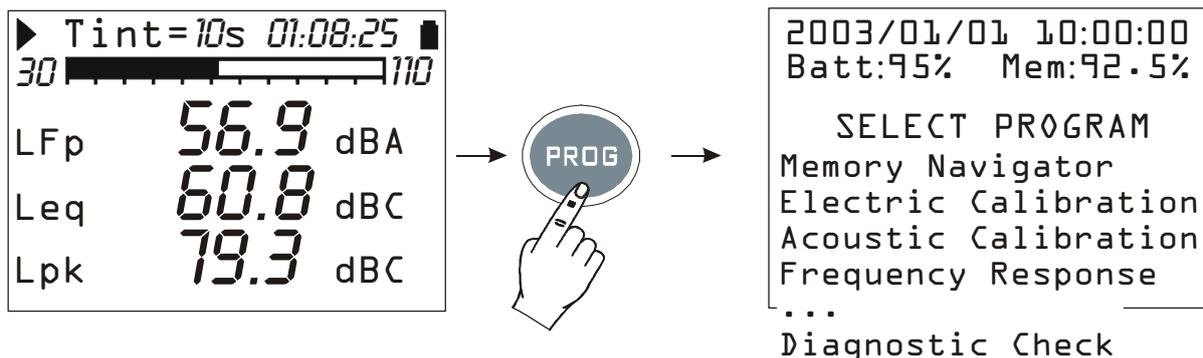
Use the UP and DOWN arrows to select the calibration to be carried out:
