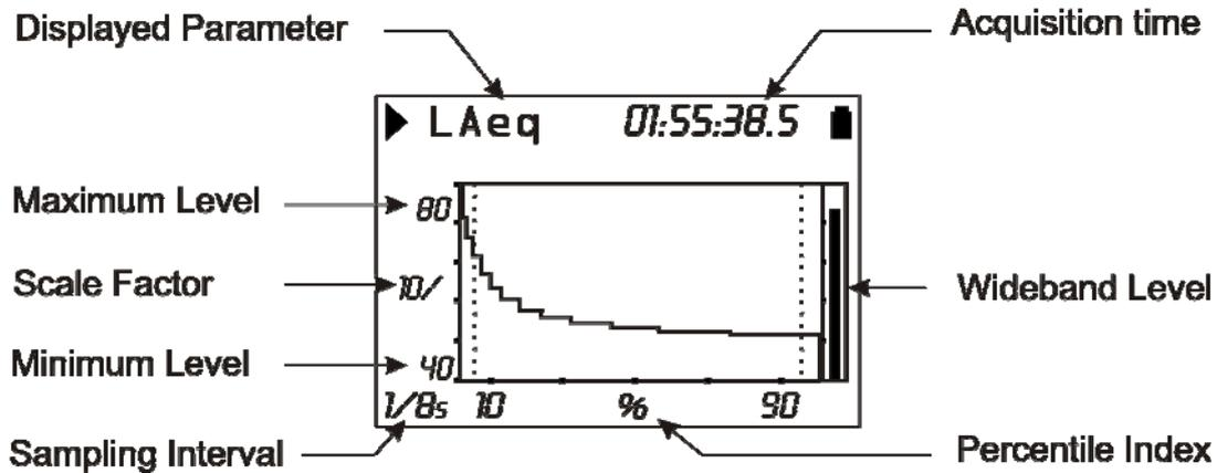
Fig. 9 - Description of the percentile levels display
