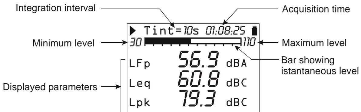
The “analogue bar” shows the **unweighted** sound pressure instantaneous level in an 80 dB interval.
