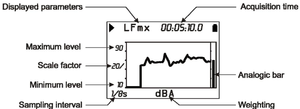
Fig. 7 - Description of the Profile mode display
