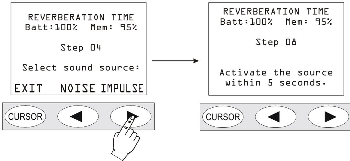
... and, as indicated in the next page, activate the impulsive noise sound source (gun shot, balloon explosion,...) **within 5 seconds** from pressing the button.
