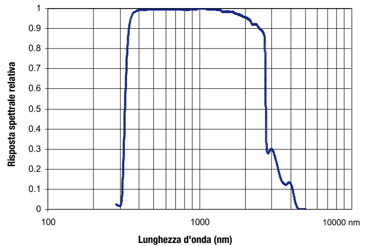
Figure 1. Typical spectral response of the pyranometers.
