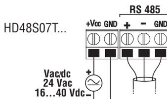
Thanks to the RS485 output, several instruments can be connected to form a network. The instruments are connected in a sequence through a shielded cable with twisted pair for signals and a third wire for the mass.
