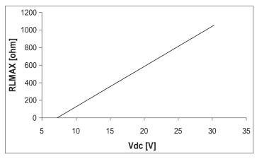
**Fig. 3** Load with relation to the supply voltage.
