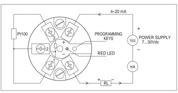
Fig. 2 Wiring diagram of the transmitters.
