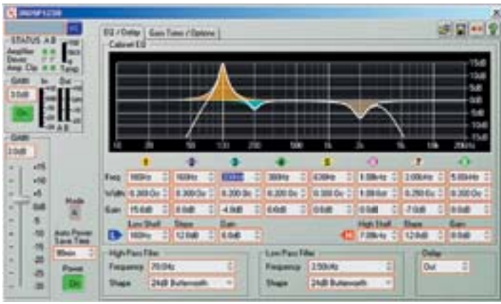
Software Podware: user defined frequency response equalization
