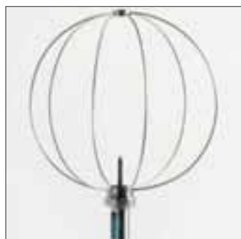
Fig.2 hot-wire probe mod. HD2001.2.
