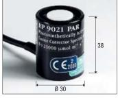
LP 9021 PAR: Quantum-radiometric probe for measuring the PHOTONS FLOW in the chlorophyll field PAR (photosynthetically Active Radiation 400nm...700nm), µmol·m<sup>-2</sup>s<sup>-1</sup> measure, cosine correction diffuser.
