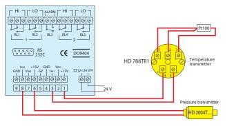
Example of connection of transmitters which are connected to the D0 9404:
