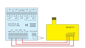
Example of connection of a passive transmitter which sends the DO 9404 two current signals (4÷20 mA)
