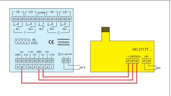
Example of connection of a self-powered transmitter which sends the DO 9404 two current signals (4÷20 mA)
