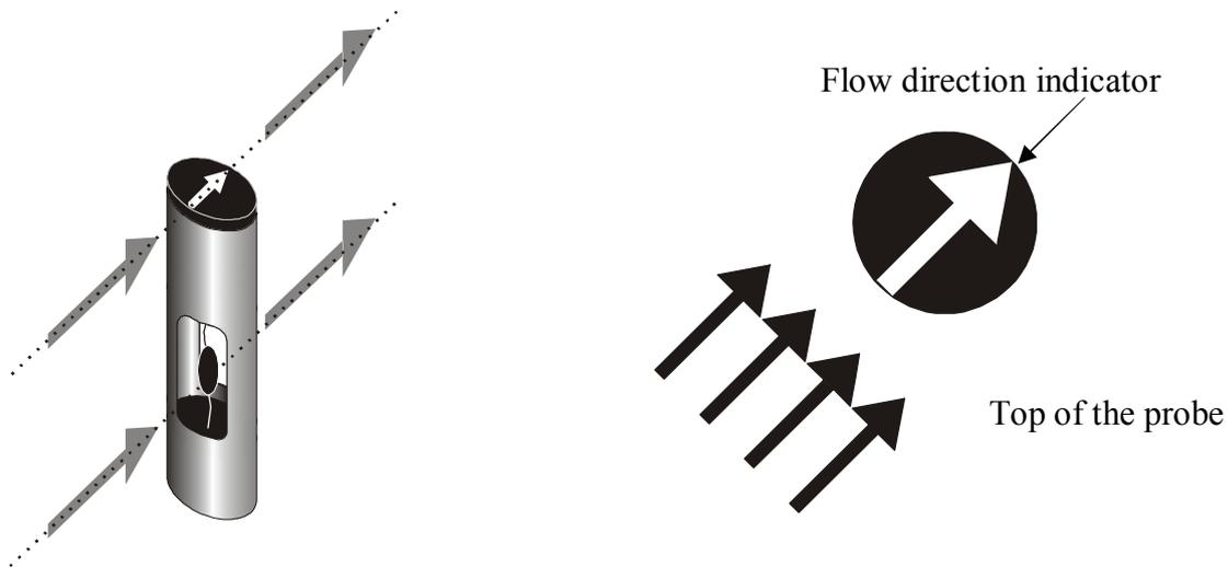
The probe should be maintained orthogonal to the flow and not tilted in relation to it:
