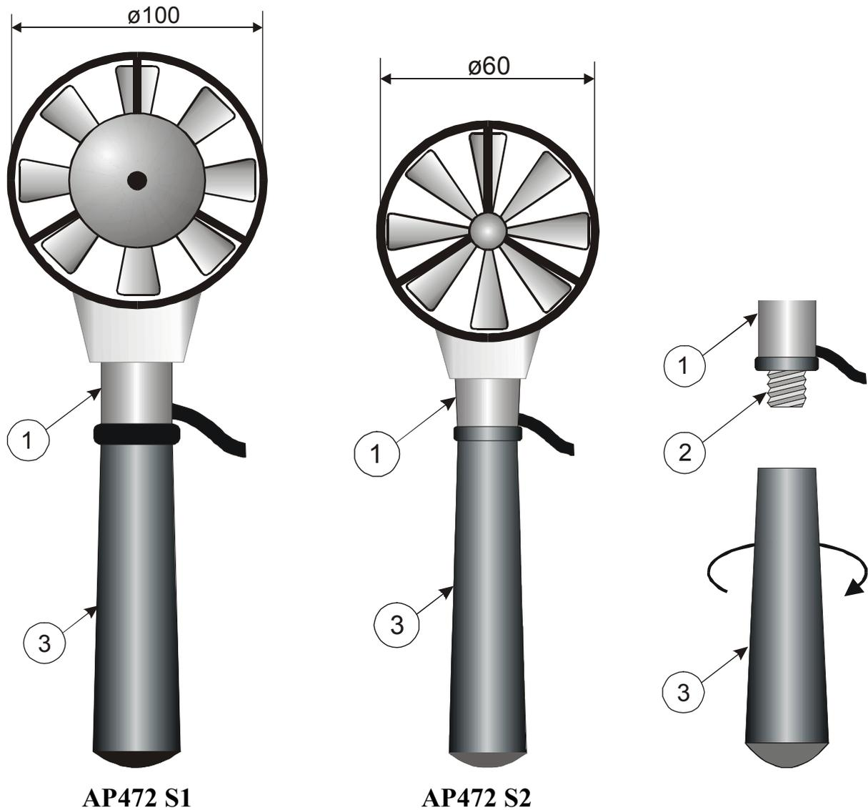
To mount the telescopic rod on the probes, unscrew the handle (3) holding the probe body still in the point (1). Screw the rod end on the screw (2). The handle (3) is screwed on the telescopic rod.
