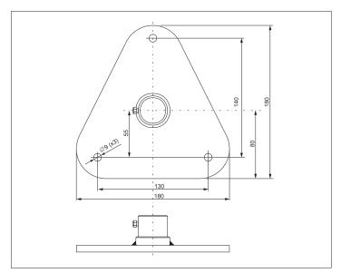
Fig. 7 - Base for installation on the floor (HD2013.78)
