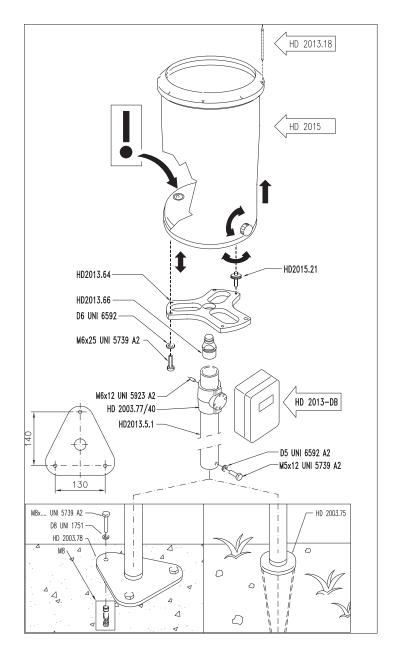
Fig. 9 - Installation off the ground
