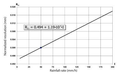
Fig. 2 - Normalized resolution (0,5 mm @ 50 mm/h as a function of the
