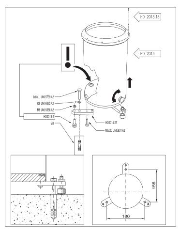
Fig. 8 - Installation on the floor
