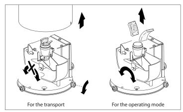
Fig. 4 - Locking and unlocking the tipping bucket
