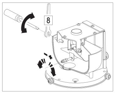
Fig. 5 - Adjustment of the tipping bucket
