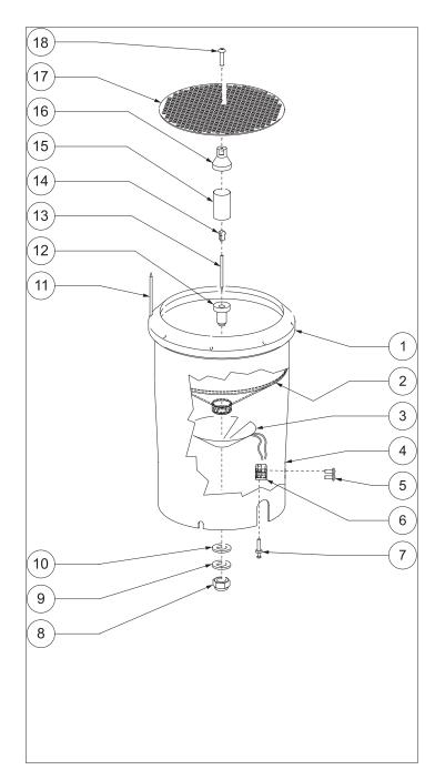
Fig. 11 - Exploded view of the upper part (version with heating system)
