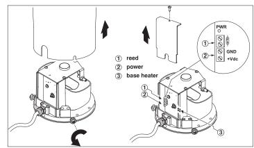
Fig. 3 - Electrical connections (version with heating system)
