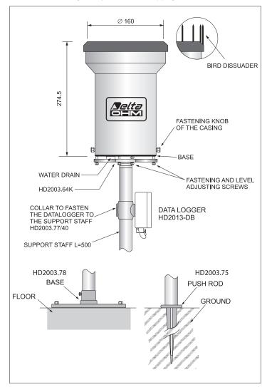
Fig. 6 - Mechanical dimensions, installation modes
